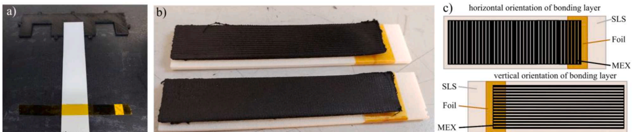
Fig. 1. (a) Position and fixture of the SLS plates, (b) ready to test SLB samples, and (c) orientations of the bonding layer.
