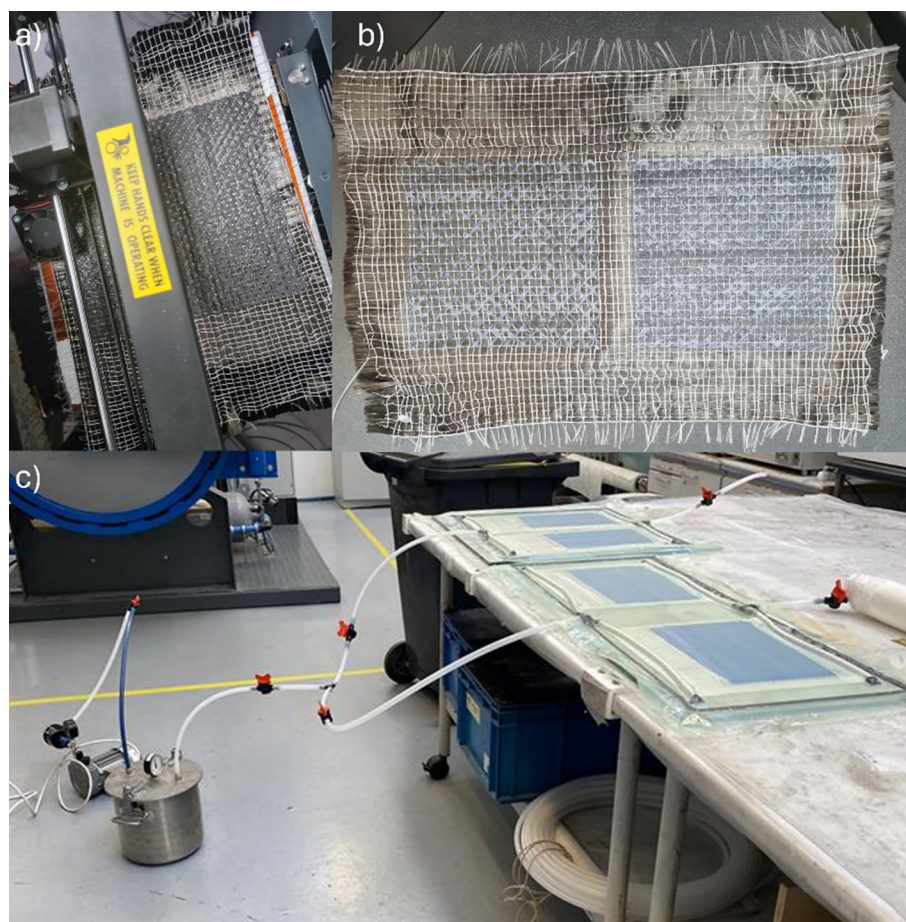
FIGURE 2 | Illustration of the fabrication process: (a) printing of the PCL interlayer onto the UD carbon fiber reinforcement; (b) printed interlayer patterns with 50% and 75% infill; (c) vacuum infusion process.
