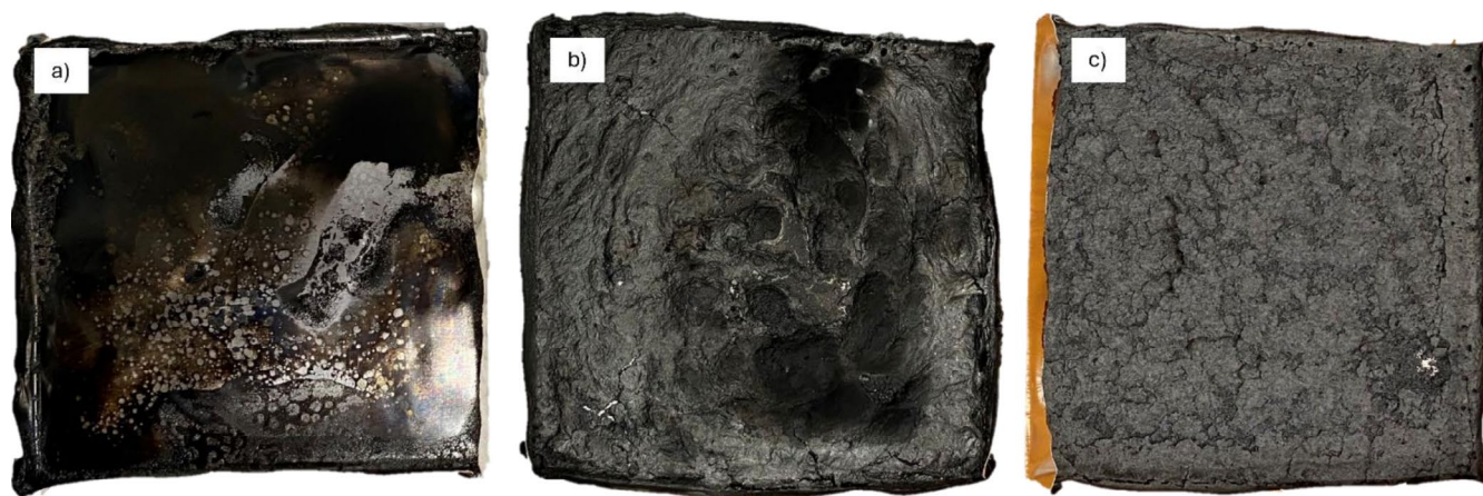
FIGURE 6 | The residues remaining after cone calorimeter testing: (a) PCL, (b) PCL_10%APP, (c) PCL_5%EG.
